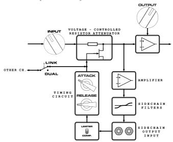
The FET compressor is fed by INPUT knob. There is no threshold or ratio setting, so the more signal gets into the compressor, the more gain reduction occurs. However, there are traditional attack / release setting knobs, allowing you to set fast to slow attack time (0.1 ms - 100 ms), and release time between 15ms to 1.5 sec. This is useful to shape the compressor's behavior and allows to use for example fast attack/release times for drums, and slower settings for vocals.
